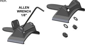
The Body Assembly must be removed to gain access to the CLAMP SCREW. Remove the two socket head screws as shown below. Be sure to remove the lock washer with the top screw along with the lock washer and flat washer with the bottom screw. Loosen the CLAMP SCREW so there is enough. clearance between the TOP and MID SECTIONS to slide over the mirror stem.
