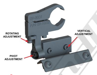
Reinstall the body assembly. Be sure to include all lock washers with screws, and the lock and flat washer with the bottom socket head screw. Use the adjustments shown above to adjust the RD to you NOTE: there are extra lock and flat washers included in the tool kit just in case you happen to misplace one.
