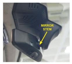
While sitting in the passenger seat, place the mount over the mirror stem. Tighten the CLAMP SCREW until the mount starts to clamp onto the mirror stem. Position the mount as far forward as it will go and paralell to the bottom of the mirror before fully tightening.
