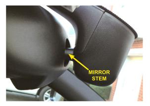
While sitting in the passenger seat, place the mount over the mirror stem. Tighten the CLAMP SCREW until the mount starts to clamp onto the mirror stem. Position the mount as far forward as it will go and paralell to the bottom of the mirror before fully tightening.
