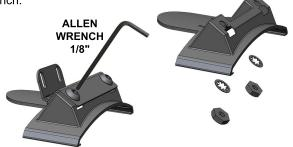
The Body Assembly must be removed to gain access to the CLAMP SCREW. Remove the two socket head screws as shown below. Be sure to remove the lock washer with the top screw along with the lock washer and flat washer with the bottom screw.
