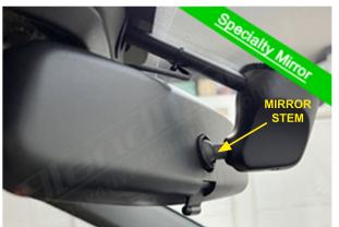
While sitting in the passenger seat, place the mount over the mirror stem. Tighten the CLAMP SCREW until the mount starts to clamp onto the mirror stem. Position the mount as far forward as it will go and parallel to the bottom of the mirror before fully tightening.
