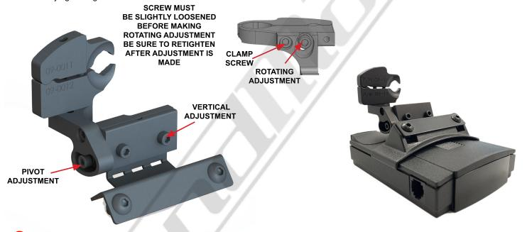
6 Install your radar detector onto the mount. Use the adjustments shown above to adjust the RD to your desired position. We recommend adjusting the RD as close to the bottom of your mirror as you can. Be sure to tighten the vertical and pivot adjustment screws after the adjustments are made. For the Pivot adjustment, grab the long arm of the allen wrench for maximum leverage. You will not strip the threaded holes in the aircraft grade aluminum.
