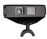
5 - Remove the bottom half of the shaft collar. This mount comes pre-assembled with a 1/2" long spacer between the angle and the shaft collar. In most applications the 1/2" long spacer is used. If a longer spacer height is needed, there is also a 3/4" long spacer included. If a shorter height is needed, use the 1/4" long screw to attach the angle directly to the shaft collar using no spacers.
