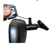
6 - Place the mount onto the mirror stem. This will allow you to determine the bends that need to be made to the angle bracket via the perforations BEFORE it is attached to the mirror. DO NOT bend the angle if it is attached to rear view mirror as this will put excessive force on the mirror and may break away from the winshield!
