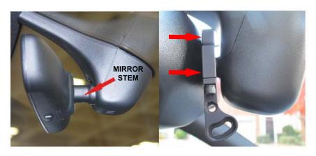
STEP 3 - While sitting in the passenger seat, place the mount over the mirror stem. Tighten the CLAMP SCREW until the mount starts to clamp onto the mirror stem. Position the mount as far forward as it will go and paralell to the bottom of the mirror before fully tightening.
