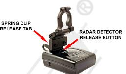
2 - Push the RD release button when installing and removing the RD onto the spring clip. Slide the clip into the RD as far as possible. Install the RD a few times so you can observe how the spring clip functions. When used properly, the spring clip avoids putting excessive pressure on the mirror stem when installing and removing the RD.
