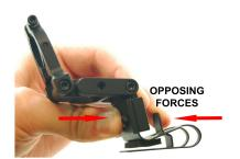
1 - Install your radar detector (RD) onto the mount before installing it on the rear view mirror. To release tension from the spring clip, simply squeeze the release tab and the back side of the mount together. This will lower the bottom portion of the spring clip allowing you to slide the RD on and off the mount.
