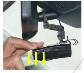
9 - To access the buttons of the RD you will need to gently push downward on the front of the RD with one finger and push the desired button with another finger. Then allow the RD to return to it's original position by gently letting it spring upward. When accessing the buttons, be sure to push the RD downward just enough for your finger to fit between the RD and mirror. Do not push down more than what is needed.
