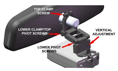
7 - Install the RD onto the mount. Make the necessary adjustments as shown above. Using the vertical adjustment, we recommend you adjust the RD as close to the bottom of the mirror as possible. The spring clip holding the RD is designed to flex downward to allow access to the RD buttons as shown below in step 9.
