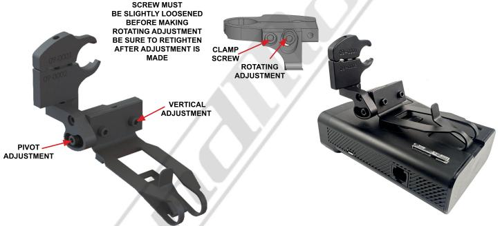
Install your radar detector onto the mount. Use the adjustments shown above to adjust the RD to your desired position. We recommend adjusting the RD as close to the bottom of your mirror as you can. Be sure to tighten the vertical and pivot adjustment screws after the adjustments are made. For the Pivot adjustment, grab the long arm of the allen wrench for maximum leverage. You will not strip the threaded holes in the aircraft grade aluminum.
