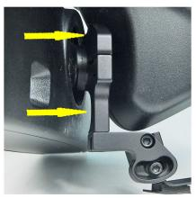
While sitting in the passenger seat, place the mount over the mirror stem. Tighten the CLAMP SCREW until the mount starts to clamp onto the mirror stem. Position the mount as far forward as it will go and parallel to the bottom of the mirror before fully tightening.
