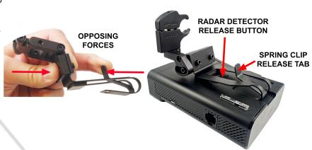
2 Loosen the CLAMP SCREW so the TOP section seperates from the MID section. This will provide the necessary clearance to slide the mount over the mirror stem as shown below. Adjust the mirror parallel to the windshield and slightly upward for ease of installation.
