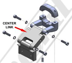
5 - The center-link may be removed if an overall shorter mount length is needed, depending on your rear view miror and desired position for the RD. With multiple adjustments available, you should be able to postion your RD right where you want it. If you are unable to achieve this, be sure to contact us at 1-707-664-8234
