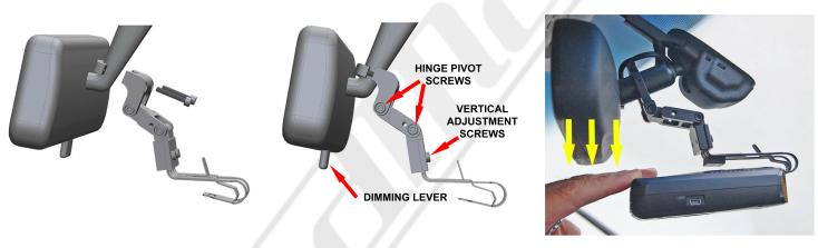
3 - Install the mount while sitting in the passenger side of your vehicle. Remove the two socket head screws so the top portion of the mount may be removed. Position the mount on the bottom of the stem as shown above. Reattach the top portion of the mount. Tighten both screws evenly making sure it is in the correct position as shown above. Tighten both screws until mount is securely attached to the mirror stem.
