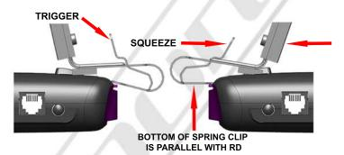
2 - The bottom of the spring clip must be parallel with the top of the RD to slide in and out. SLIDE THE RD ONTO THE SPRING CLIP AS FAR AS IT WILL GO. Release the trigger to secure the RD onto the mount. Before installing the mount onto your rear view mirror, remove and install the RD a few times so you can observe how the spring clip functions.
