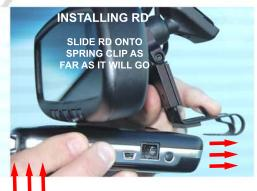
7 - When removing or installing the RD, squeeze the trigger and the back side of the mount together with one hand, and lift the front of the RD upward with the other hand before sliding the RD off or onto the spring clip. You must lift the front of the RD upward before sliding it off or onto the mount.
