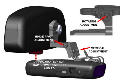
5 - Install the RD onto the mount. Make the necessary adjustments as shown above. Using the vertical adjustment, we recommend you adjust the RD so there is approximately 1/2" gap between the bottom of the mirror and the top of the RD. After all adjustments are made, be sure to check that all adjustment screws are tight. Grab the long arm of the allen wrench to assure that these screws are securely tightened. You will not strip out the tapped holes in the aircraft grade aluminum.
