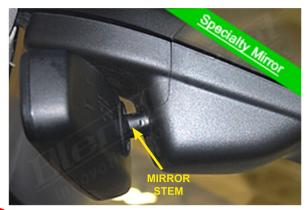
While sitting in the passenger seat, place the mount over the mirror stem. Tighten the CLAMP SCREW until the mount starts to clamp onto the mirror stem. Position the mount as far forward as it will go and paralell to the bottom of the mirror before fully tightening.
