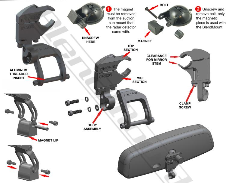
Install aluminum threaded insert into magnet, and attach magnet onto blendmount with lip pointed in direction as shown.
