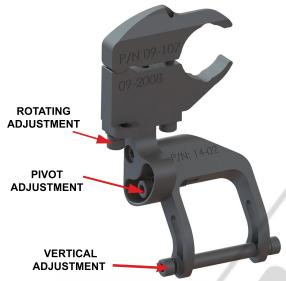
Reinstall the body assembly. Be sure to include all lock washers with screws, and the lock and flat washer with the bottom socket head screw as shown above. Use the adjustments shown above to adjust the RD to your desired position. We recommend adjusting the RD as close to the bottom of mirror as possible. Be sure to tighten all screws after adjustments are made.
