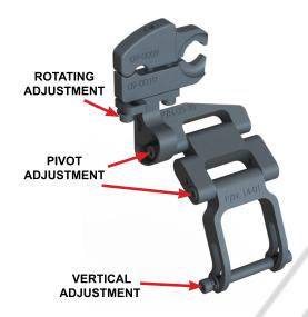
Reinstall the body assembly. Be sure to include all lock washers with screws, and the lock and flat washer with the bottom socket head screw as shown above. Use the adjustments shown above to adjust the RD to your desired position. We recommend adjusting the RD as close to the bottom of mirror as possible. Be sure to tighten all screws after adjustments are made.
