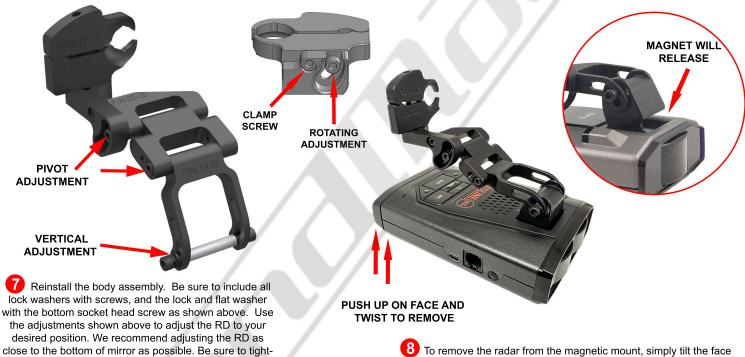
To remove the radar from the magnetic mount, simply tilt the face of the RD up and twist slightly to side, then the magnet will release.
