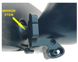
While sitting in the passenger seat, place the mount over the mirror stem. Tighten the CLAMP SCREW until the mount starts to clamp onto the mirror stem. Position the mount as far forward as it will go and paralell to the bottom of the mirror before fully tightening.
