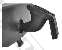
Reattach right side of the mount. Make sure small lock washer is still on lower screw and tighten until fairly snug. Leave top screw loose so mount can slide towards windshield around the large diameter of the mirror stem. Slide the mount upwards leaving approximately 1/8" of clearance between mount and the windshield. Rotate mount until level from side to side and tighten the top screw.
