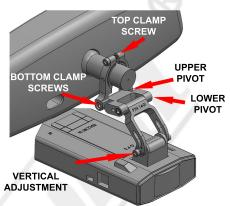
Install the RD onto the mount. Make the necessary adjustments as shown above. Using the upper and lower pivots, and the vertical adjustment, leave enough room below bottom of mirror to allow access to buttons on top of radar detector.
