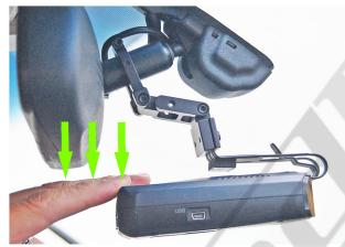
**STEP 6** - If the RD is too close to the bottom of the mirror, You may access the buttons on top of the RD by gently pushing downward on the front of the RD with one finger and push the desired button with another finger. Then allow the RD to return to it's original position by gently letting it spring upward. When accessing the buttons, be sure to push the RD downward just enough for your finger to fit between the RD and mirror. **Do not push down more than what is needed.**
