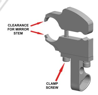
STEP 3 - BEFORE FULLY TIGHTENING THE CLAMP SCREW, POSITION THE MOUNT AS FAR FORWARD TO-WARDS THE WINDSHIELD AS YOU CAN. MAKE SURE THE TOP AND MID SECTIONS ARE TOUCHING AT THE PIVOT POINT. If you can not get them to touch at the pivot point, you have an incompatible mirror type for this mount.
