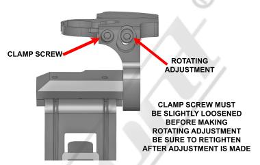
STEP 5 - Use adjustments shown to install RD to your desired position. We recommend adjusting RD as close to bottom of mirror as possible. Be sure to tighten vertical and pivot adjustment screws after adjustments are made. For Pivot adjustment, grab long arm of allen wrench for maximum leverage. You will not strip the threaded holes in the aircraft grade aluminum.
