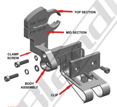
STEP 2 - Loosen the CLAMP SCREW so there is enough clearance between the TOP and MID SECTIONS to slide over the mirror stem.
