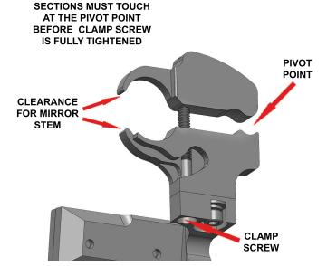
STEP 3 - BEFORE FULLY TIGHTENING THE CLAMP SCREW, POSITION THE MOUNT AS FAR FORWARD TO-WARDS THE WINDSHIELD AS YOU CAN. MAKE SURE THE TOP AND MID SECTIONS ARE TOUCHING AT THE PIVOT POINT. If you can not get them to touch at the pivot point, you have an incompatible mirror type for this mount.
