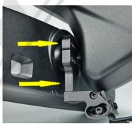
4 - Rotate the mount so it is parallel with the bottom of the mirror. Tighten the clamp screw untill the mount is securely attached to the mirror stem.
