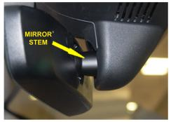
3 - When the mount is positioned as far forrward as it will go, tighten the clamp screw untill the Top and Mid Sections are slightly snug around the mirror stem. You should still be able to rotate the mount.
