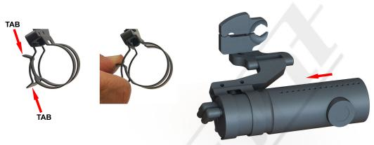
1 - To install the dashcam into the mount, simply squeeze the two tabs of the spring clip together as shown above. This will increase the diameter of the spring clip and allow you to slide the dashcam into position. Once the dashcam is in position, release the two tabs. The dashcam is now securely attached to the mount.
