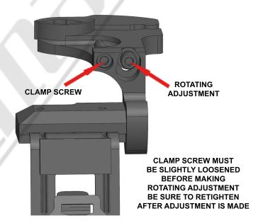
STEP 5 - Install your radar detector onto the mount. Use the adjustments shown above to adjust the RD to your desired position. We recommend adjusting the RD as close to the bottom of your mirror as you can. Be sure to tighten the vertical and pivot adjustment screws after the adjustments are made. For the Pivot adjustment, grab the long arm of the allen wrench for maximum leverage. You will not strip the threaded holes in the aircraft grade aluminum.
