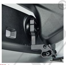
**STEP 4 -** Rotate the mount so it is parallel with the bottom of the mirror. Tighten the clamp screw untill the mount is securely attached to the mirror stem. Do not over tighten the clamp screw.
