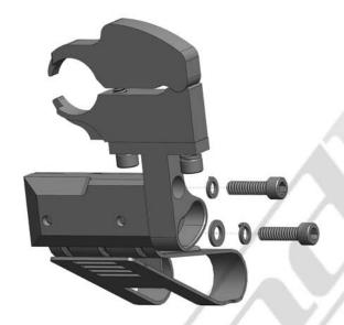
STEP 5 - Reinstall the BODY ASSEMBLY. Be sure to include the lock washer with the top socket head screw and the lock and flat washer with the bottom socket head screw as shown above. NOTE: there are extra lock and flat washers included in the tool kit just in case you happen to misplace one.
