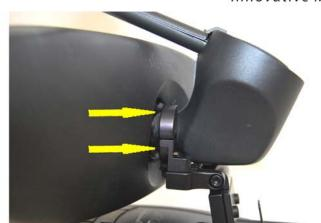
STEP 3 - When the mount is positioned as far forrward as it will go, tighten the clamp screw untill the Top and Mid Sections are slightly snug around the mirror stem. You should still be able to rotate the mount.
