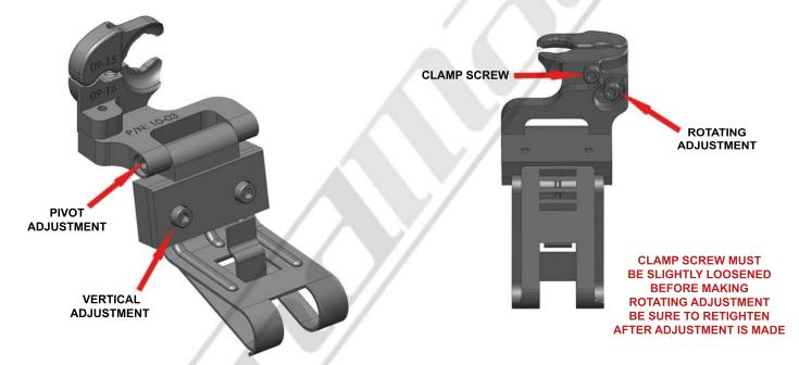
STEP 5 - Install your radar detector onto the mount. Use the adjustments shown above to adjust the RD to your desired position. We recommend adjusting the RD as close to the bottom of your mirror as you can. Be sure to tighten all adjustment screws after the adjustments are made. For the Pivot adjustment, grab the long arm of the allen wrench for maximum leverage. You will not strip the threaded holes in the aircraft grade aluminum.
