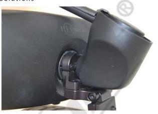
**STEP 4** - Rotate the mount so it is parallel with the bottom of the mirror. Tighten the clamp screw untill the mount is securely attached to the mirror stem.
