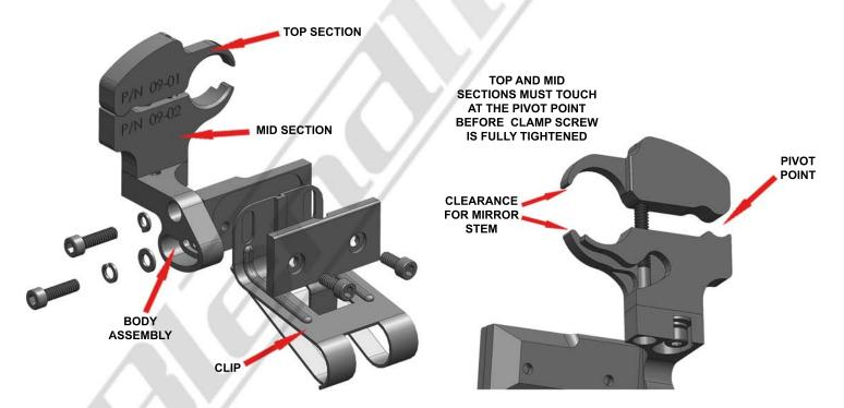
STEP 1 - Loosen the clamp screw so the top section seperates from the mid section. This will provide the necessary clearance to slide the mount over the mirror stem as shown above. Adjust the mirror paralell to the windshield and slightly upward for ease of installation.
