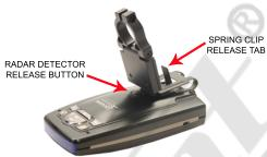
2 - Push the RD Release button and slide the RD onto the Spring Clip until the RD hits the bottom of the Tab. Then release both the Tab and the Button. Now slide the RD toward you until you hear it lock into position. Remove the RD a few times so you can observe how the spring clip functions. When used properly, the spring clip avoids putting excessive pressure on the mirror stem when installing and removing the RD.
