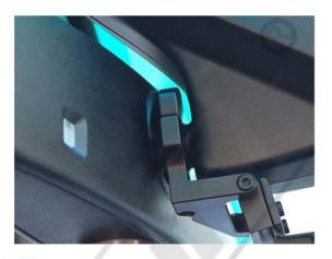
**STEP 6** - Rotate the mount so it is parallel with the bottom of the mirror. Tighten the clamp screw untill the mount is securely attached to the mirror stem. Do not over tighten the clamp screw.
