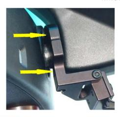
STEP 5 - Position the mount as far forward as you can. Tighten the clamp screw untill the Top and Mid Sections are slightly snug around the mirror stem. You should still be able to rotate the mount.
