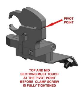
STEP 4 - BEFORE FULLY TIGHTENING THE CLAMP SCREW, MAKE SURE THE TOP AND MID SECTIONS ARE TOUCHING AT THE PIVOT POINT. If you can not get them to touch at the pivot point, you have an incompatible mirror type for this mount.
