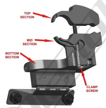
STEP 3 - Loosen the clamp screw so the top section seperates from the mid section. This will provide the necessary clearance to slide the mount over the mirror stem as shown above. Adjust the mirror parallell to the windshield and slightly upward for ease of installation.
