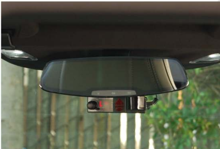
The pictures above show the vertical adjustment set to where the RD can be removed from the mount without hitting the bottom of the mirror.
