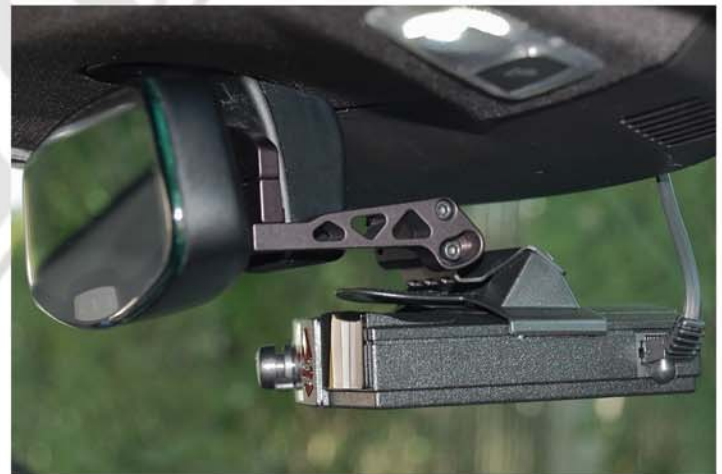
The pictures above show the vertical adjustment set to where the RD can be removed from the mount without hitting the bottom of the mirror.
