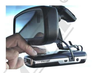
6 - To access the buttons of the RD you will need to gently push downward on the front of the RD with one finger and push the desired button with another finger. Then allow the RD to return to it's original position by gently letting it spring upward. When accessing the buttons, be sure to push the RD downward just enough for your finger to fit between the RD and mirror. Do not push down more than what is needed.
