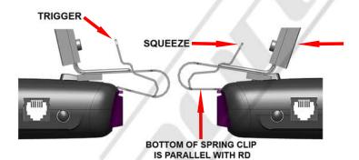
1 - The RELEASE Button on the radar detector (RD) is NOT used with this mount. To release the tension of the spring clip, simply squeeze the TRIGGER and the back side of the mount together. This will lower the bottom portion of the spring clip allowing you to slide the RD on and off. When used properly, the spring clip avoids putting excessive pressure on the mirror stem when installing and removing the RD. The top portion of the mount should barely move when the two opposing forces are applied.
