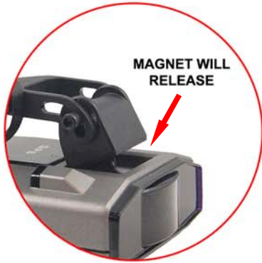
6 - Install the RD onto the mount. Make necessary adjustments using the upper and lower pivots, and the vertical adjustment. Leave enough room below bottom of mirror to allow access to top radar detector buttons. To remove the radar from the magnetic mount, simply tilt the face of the RD up and twist slightly to side, then the magnet will release.
