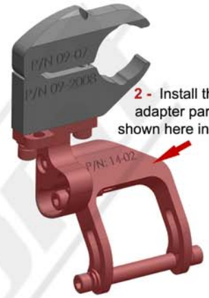
1 - Remove the three lower pieces of your existing mount, shown here in red.
