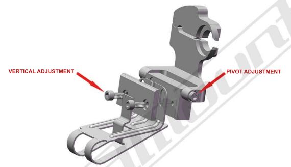
STEP 5 - Install your radar detector onto the mount. Use the adjustments shown above to adjust the RD to your desired position. We recommend adjusting the RD as close to the bottom of your mirror as you can. Be sure to tighten the vertical and pivot adjustment screws after the adjustments are made. For the Pivot adjustment, grab the long arm of the allen wrench for maximum leverage. You will not strip the threaded holes in the aircraft grade aluminum.
