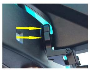
STEP 4 - Position the mount towards the front of the vehicle as far as it will go. Rotate the mount so it is parallel with the bottom of the mirror. Tighten the clamp screw untill the mount is securely attached to the mirror stem. Do not over tighten the clamp screw.
