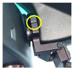
**STEP 3** - If the pivot points are touching, tighten the clamp screw untill the top and bottom pieces are slightly snug around the mirror stem. You should still be able to rotate and move the mount along the mirror stem.
