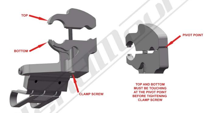
STEP 1 - Loosen the clamp screw and remove the top of the mount. Reattach the top by tightening the clamp screw just two revolutions. This will provide the necessary clearance to slide the mount over the mirror stem as shown above.
