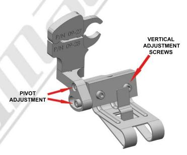
STEP 6 - Install your radar detector onto the mount. Use the adjustments shown above to adjust the RD to your desired position. We recommend adjusting the RD as close to the bottom of your mirror as you can. Be sure to tighten all adjustment screws after the adjustments are made.
