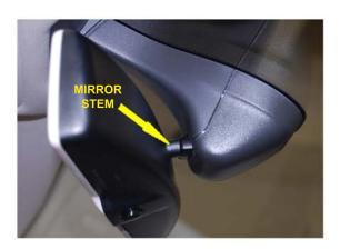
**STEP 3** - While sitting in the passenger seat, place the mount over the mirror stem. Tighten the CLAMP SCREW until the mount starts to clamp onto the mirror stem. Position the mount as far forward as it will go and paralell to the bottom of the mirror before fully tightening.
