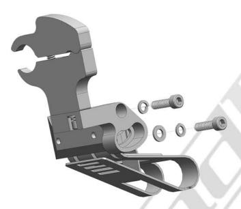
STEP 5 - Reinstall the BODY ASSEMBLY. Be sure to include the lock washer with the top socket head screw and the lock and flat washer with the bottom socket head screw as shown above. NOTE: there are extra lock and flat washers included in the tool kit just in case you happen to misplace one.
