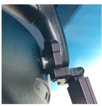
**STEP 4** - Rotate the mount so it is parallel with the bottom of the mirror. Tighten the clamp screw untill the mount is securely attached to the mirror stem.
