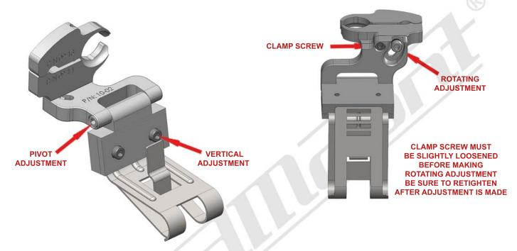
STEP 5 - Install your radar detector onto the mount. Use the adjustments shown above to adjust the RD to your desired position. We recommend adjusting the RD as close to the bottom of your mirror as you can. Be sure to tighten all adjustment screws after the adjustments are made. For the Pivot adjustment, grab the long arm of the allen wrench for maximum leverage. You will not strip the threaded holes in the aircraft grade aluminum.
