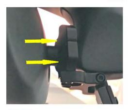
**STEP 3** - When the mount is positioned as far forrward as it will go, tighten the clamp screw untill the Top and Mid Sections are slightly snug around the mirror stem. You should still be able to rotate the mount.
